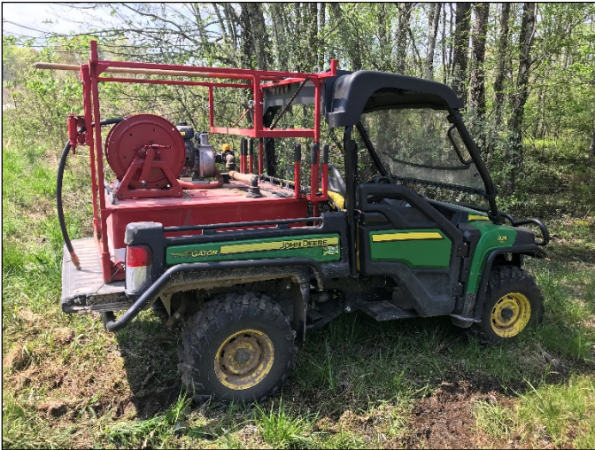
This UTV rig is equipped with a water tank, pump, and hose reel, making it a highly mobile suppression vehicle. UTVs can also haul personnel, fire tools, and drip torch fuel.
